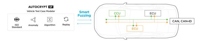
Instead of generating fully randomized packets, AutoCrypt\* Security Fuzzer analyzes the architecture and sequence of the communication protocols of the in-vehicle software, then generates test cases by randomly modifying only parts of a message that could potentially be defaced, leaving the remaining parts untouched.
